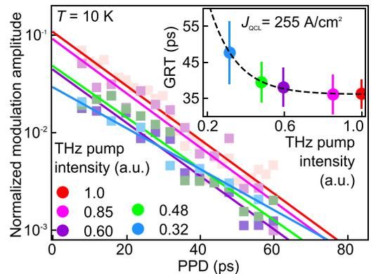
FIG. 2. The gain recovery in a THz QCL with a heterogeneous active region at several different THz-pump pulse intensities related to the maximum—for NIR pulses with 62 mW power focused on the emitter. (Dots—GRT; vertical bars—error margins; and dashed line—a guide to the eye).
