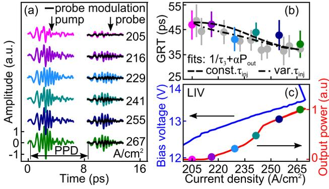
FIG. 3. The gain recovery for different driving conditions of the QCL: (a) selected time-domain THz-pump/THz-probe data for a pump-probe delay (PPD) of 8 ps (pulses are vertically offset for clarity); (b) gain recovery time as a function of the driving current density [gray dots—the time-domain data is not shown in (a)]; and (c) THz output power and QCL bias voltage as a function of driving current density.
