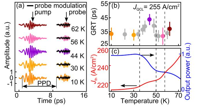
FIG. 5. Temperature dependence of the gain recovery of the THz QCL: (a) selected time-domain THz-pump/THz-probe data (pulses are vertically offset); (b) observed gain recovery time [gray dots—data not displayed in (a)]; and (c) the threshold current  $J_{th}$  and THz output power as a function of temperature.
