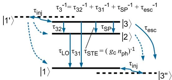
FIG. 4. Rate equation model for the THz quantum cascade heterostructure design (dashed-line arrows—direct scattering from/injector states that are neglected in the considered model).
