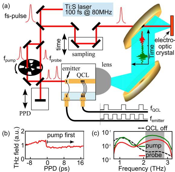
FIG. 1. THz-pump/THz-probe spectroscopy for the assessment of the gain recovery time in a THz QCL: (a) schematic of the optical setup and the modulation scheme; (b) amplitude of the THz-probe, which is generated in the integrated emitter for the THz-pump at 0 ps, is plotted as a function of the pump-probe delay time (PPD); (a) and (c) THz pulses and the spectral content of the THz pulses after the propagation through the QCL section.
